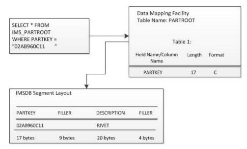
Figure 2. Using the Data Mapping Facility with the IBM Open Data Analytics for z/OS Interface for IMB DB/SQL
